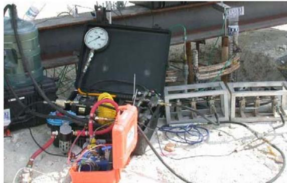
A calibrated, high-pressure bourdon gauge will be used to read the pressure on the pump line and a calibrated pressure transducer will read the pressure on the return line. Applied load is determined by relating the hydraulic pressure to the O-cell load calibration curves.
