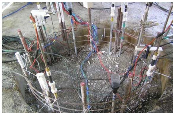
Once the instrumentation is set up and before zero readings are taken, the area should be cordoned off and any adjacent site operations which might disturb the test must be stopped.
