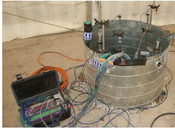
A datalogger will be used to measure and record directly data from all of the sensors from within the pile and on the pile head at intervals of 30 or 60 seconds. Data is stored in the datalogger memory and transmitted directly to the field computer for live monitoring.
