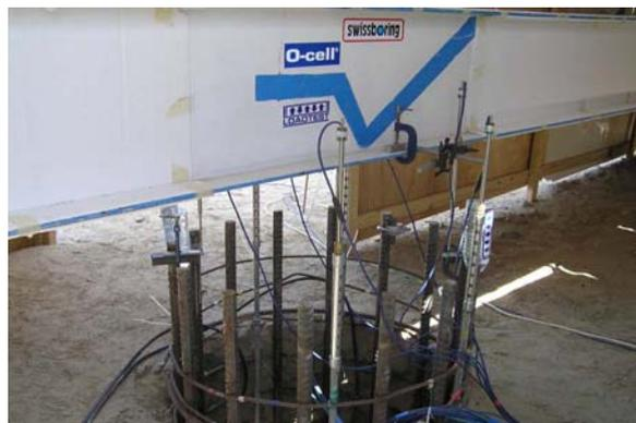
When on land, a simple reference beam can be set up using a rigid steel I-beam resting on supports at least 3 pile diameters away from the test pile. LVDTs or LVWDTs mounted on the reference beam can measure the top of pile movement.
