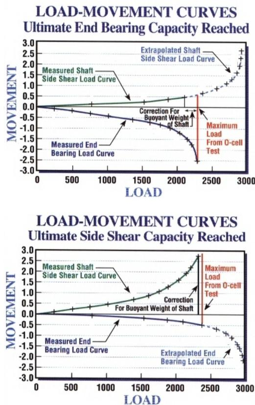
The test will start with pressurising the O-cell(s) to break the tack welds and separate the two elements of the pile. Loading steps will then be carried out according to the detailed method statement.
