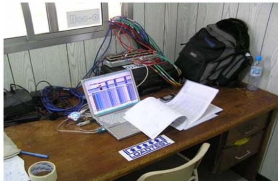
The field computer displays in real time the results from all of the sensors and records any electronic level data being measured. The computer can also control the pumps directly and allow supervision of the loading schedule according to the agreed test specification.
