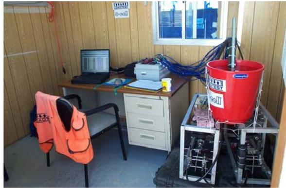
Testing is carried out from inside a cabin. The O-cell(s) will be pressurized typically with water through high pressure hydraulic pumps. Compressed air (at 100psi) is used to energize these pumps.
