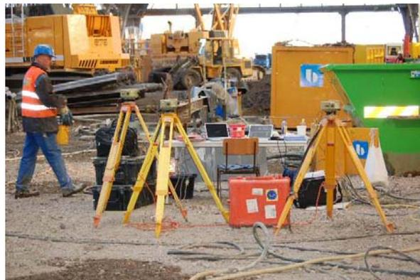
Where other site activities may disturb the reference beam or where the test is performed without the need of a reference beam over the top of the pile, multiple electronic Leica levels may be employed to monitor the top of pile movement directly and independently.
