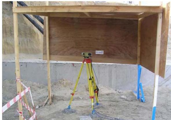
In addition to the reference beam, an additional independent optical electronic system is used to monitor the reference beam movement automatically from a more remote location. (between 5-20m). Shading of the instrument should be provided.
